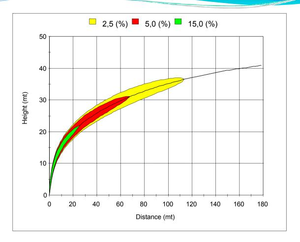
Leakage Sample 2: Natural gas release DN100 - 0,5 barg - 20 °C Meteo: wind 2 m/s Less wind speed means a lower dispersion and dilution with higher concentration till long distance from the emission point
