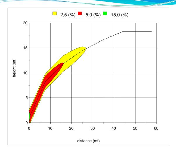
Leakage Sample 1: Natural gas release DN100 - 0,5 barg - 20 °C Meteo: wind 5 m/s Gas density is lower than the atmosphere and it is venting free.
