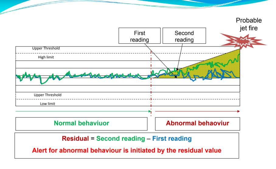
A continuous comparison between the data recorded by each single flow meter is also integrated by a continuous comparison between the data read and recorded in the previous cycle. The difference or better the residual is detected as an abnormal condition if out of the thresholds and a probable Jet Fire.
